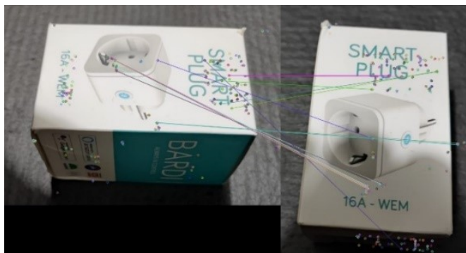
Figure 6. ORB algorithm matching result
