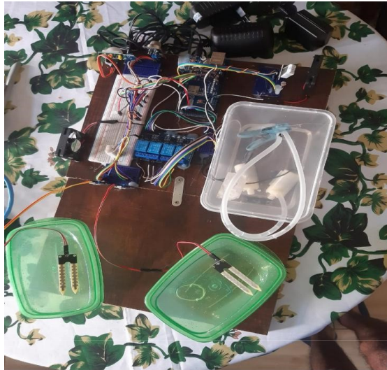
Figure. 3. Arduino mega board with the sensors, ethernet shield and relay
